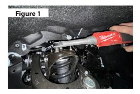
2. Loosen, but DO NOT remove the lower control arm mounting bolts.
