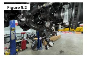
**6.** Remove the strut from the vehicle.
