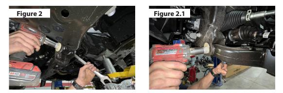
**3.** Remove the sway bar mounting bolts on the driver and passenger side frame. Let the sway bar hang loosely.
