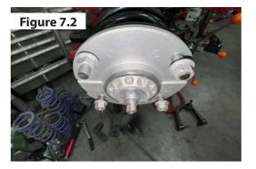
**8.** Locate and install one of the new upper strut spacers on the top of the OE strut using the OE nuts.
