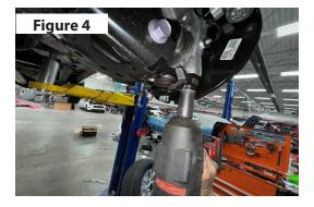
5. Remove the lower strut mounting bolt and hardware from the lower control arm.
