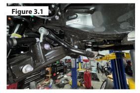
**4.** Working on the driver side, Remove the (2) bolts holding the lower ball joint mount to the knuckle. Save hardware.
