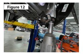
**13.** Move back to the 4 new 3/8" flange nuts on top of the strut and torque to 40 ft lbs.
