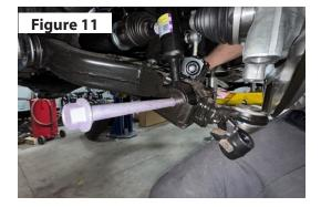
**12.** Re-install the 2 lower ball joint mounting bolts to the bottom of the steering knuckle. Torque to 150 ft lbs.
